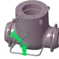
Bypass and Equalizing (Unidirectional)
